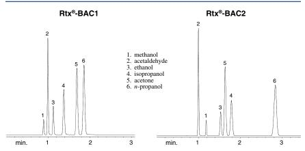
30m, 0.53mm ID, 3.0μm Rtx-BAC1 (cat.# 18001) 30m, 0.53mm ID, 2.0μm Rtx-BAC2 (cat.# 18000) 1.0mL headspace sample of a blood alcohol mix. Sample conc. 0.1% per compound.
