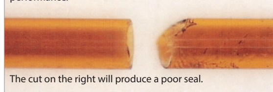
Figure 1: Make a clean, square cut for optimum connector performance.
