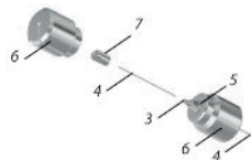
Figure 3: Exploded view of installing the female \mu -connector end fitting.
