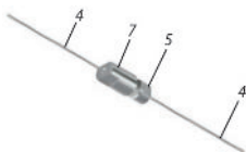
Figure 6: Completed SiTite \mu -Union connection.
