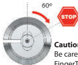
Figure 7: Do not overtighten \mu -connector end fittings.
