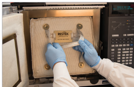
Figure 6: Only remove the plate insert once the system has sufficiently cooled.
