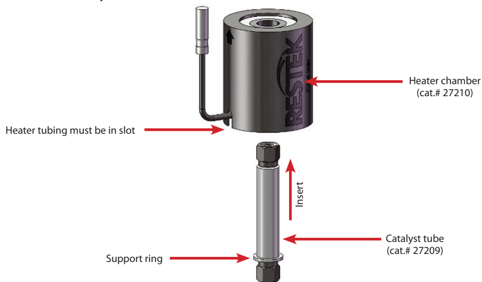
Figure 5: Heater Chamber and Catalyst Tube
