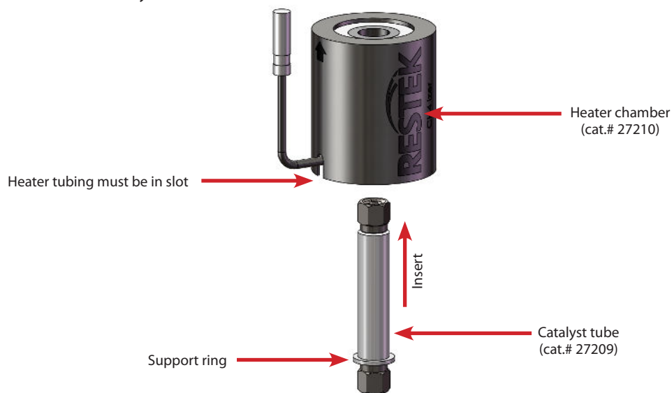
Figure 4: Heater Chamber and Catalyst Tube
