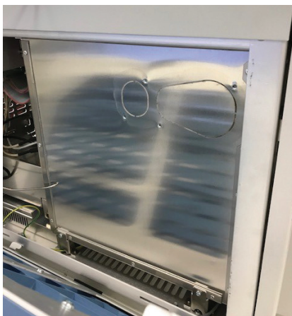
Figure 3: Removing GC Oven Cutout and Insulation
