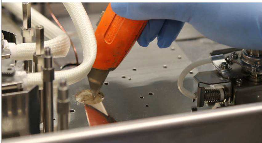
Figure 3: Removing GC Oven Cutout and Insulation
