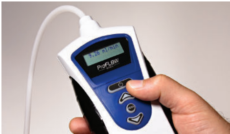
Figure 5: LED displays the measured flow value.
