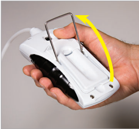
Figure 2: Extend the wire stand before opening battery door.
