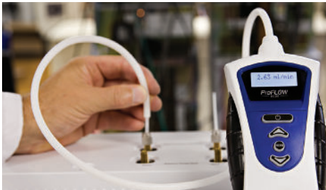
Figure 4: Probe connected to a GC gas outlet.
