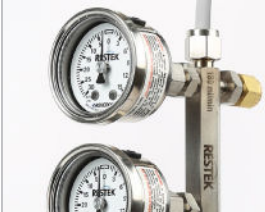
Figure 3: A sample line installed in the sample inlet of a soil gas sampler.
