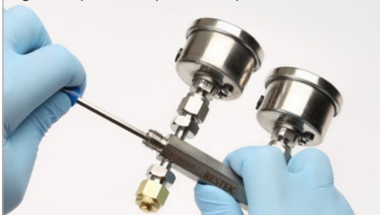
Figure 5: Open the sample inlet to replace the frit.
