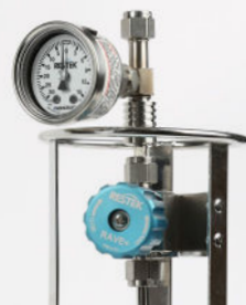
Figure 4: Open the sample inlet to replace the frit.
