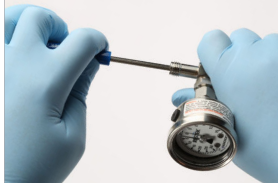
Figure 4: Open the sample inlet to replace the frit.
