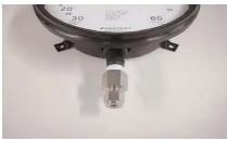
**4.** Wrap three layers of PTFE tape around the threads on the gauge. Thread the female connector onto the gauge and tighten.
