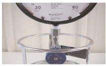
5. Finally, slide the gauge with the female connector attached onto the port connector and tighten ¼ turn past finger-tight. You are now ready to open the valve and take vacuum and pressure readings.
