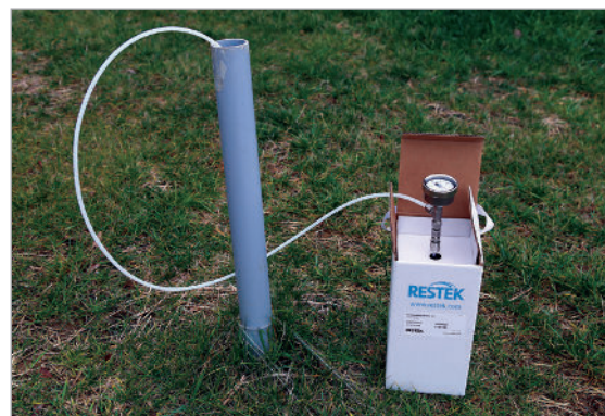
Figure 1: Direct access to the quick-connect valve allows the air sampling bottle to remain in its protective packaging during use, preventing bottle breakage and sample loss.
