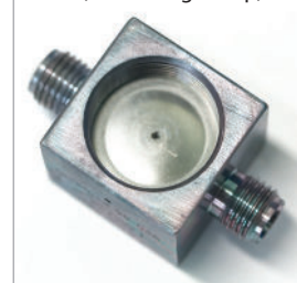
Figure 3: Preassembled diaphragm stack installed in valve (black dot goes up).
