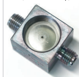
Figure 3: Preassembled diaphragm stack installed in valve (black dot side up).
