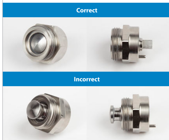
Figure 6: The stem must be fully threaded (retracted) into the bonnet nut before the bonnet nut/stem assembly is installed or the valve may be damaged during installation.
