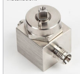
Figure 7: Bonnet nut/stem assembly installed on valve. Orient the channel and pin correctly prior to knob installation.
