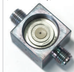
Figure 5: Button installed into bonnet inside of valve (black dot side up).
