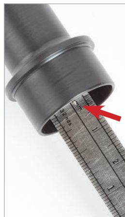
Figure 9: Exposure Depth for Headspace Extraction
