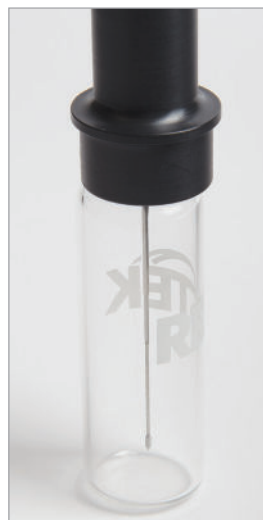
Figure 13: Distance from Lower Groove of the Adaptor Cup to Tip of SPME Arrow or SPME Fiber
