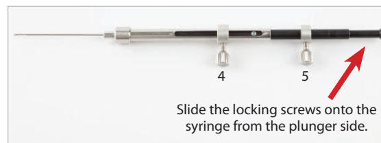
Figure 4: Attaching the Locking Screws to the Syringe
