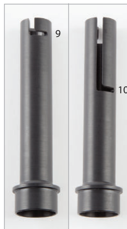
Figure 7: Proper Positioning of a SPME Arrow in the Extraction Guide
