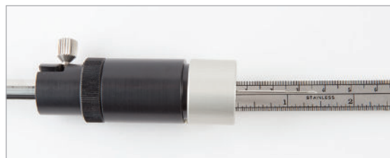
Figure 14: Adjusting the Desorption Depth
