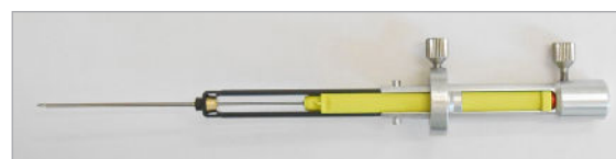
Figure 4: The Smart SPME Arrow Inserted and Fixed in the Manual Smart SPME Arrow Holder
