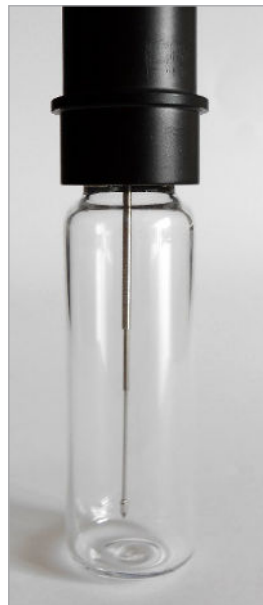
Figure 14: Maximum adjustable penetration depth of 70 mm
