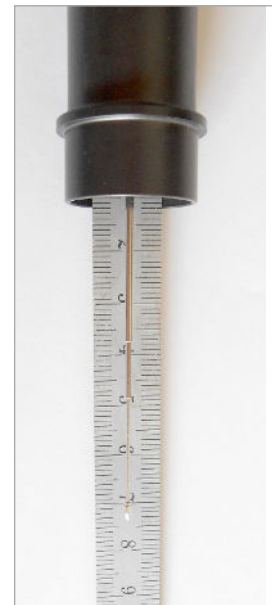
Figure 14: Maximum adjustable penetration depth of 70 mm
