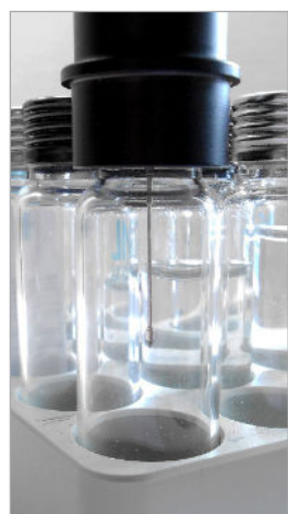
Figure 10: Determine the optimum penetration depth directly in a vial.
