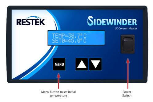
Turn the column heater on. The temperature controller will perform a self-diagnostic test upon power up. If, after powering up, the display indicates something other than reasonable temperature values, notify technical service@restek.com for further action.
