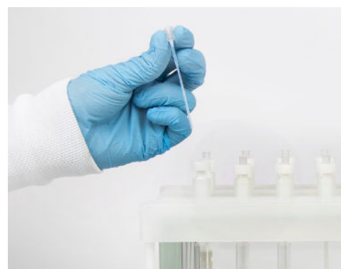
Figure 3: Disposable Resprep Quick-Replace valve liners provide a clean, continuous flow path that is easily replaced between samples to eliminate contamination.
