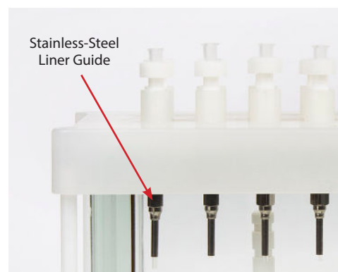
Figure 2: A Properly Installed Stainless-Steel Liner Guide
