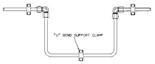
Figure 22 U-Bend Allowing for Expansion and Contraction
