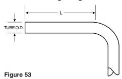
**Note:** You will need a minimum straight length of tubing ahead of any bend to fit into the presetting tool. See the "L" dimension in the chart for each tube O.D. size.
