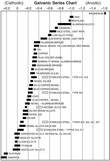
Above represents corrosion potentials of materials in flowing seawater at temperature in the range 10°C – 26°C. The hatched symbols indicate potentials exhibited by stainless steels in pits or crevices.
