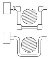
**Figure 1** Tubing provides simplified, free flow system.
