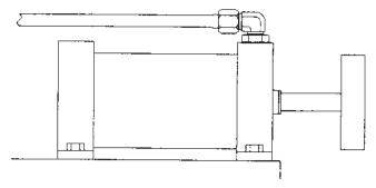
Figure 23 Bent Tube Allowing for Motion Under Load
