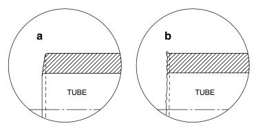
**Figure 30** Enlarged section of tube showing differences in tubing cut with a tube cutter (a) and a hacksaw (b).
