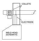
Figure 62 – The orbital welded electrode is shielded within the mini-weld head and rotates 360° to produce uniform, accurate, 100% penetration welds.
