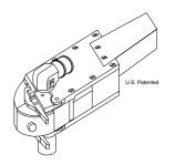
**Figure 58** The orbiting electrode is precisely positioned over the end collar by engaging the locator rib within the weld head.
