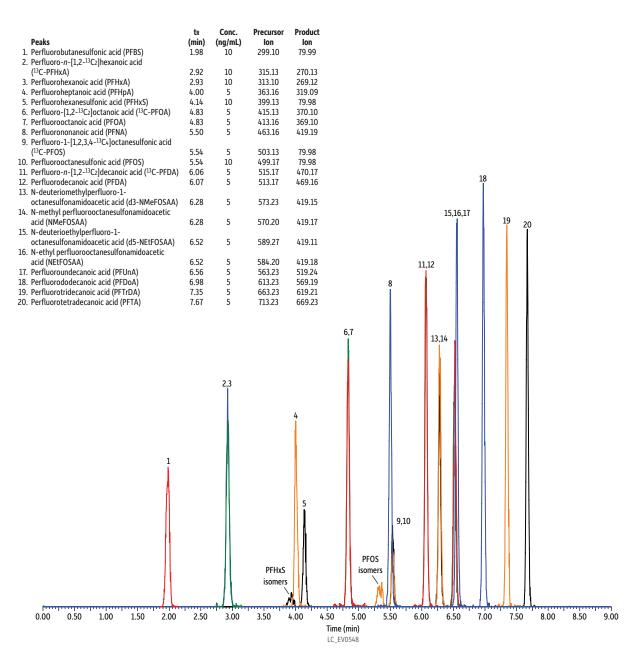
Column: Raptor C18 (cat.# 9304552); Dimensions: 50 mm x 2.1 mm ID; Particle Size: 5 µm; Pore Size: 90 Å; Temp.: 40 °C; Sample: Diluent: 96:4 Methanol:water; Conc.: 5–10 ng/mL; Inj. Vol.: 2 µL; Mobile Phase: A: 5 mM ammonium acetate in water; B: Methanol; Gradient (%B): 0.00 min (25%), 8.00 min (85%), 8.01 min (25%), 9.00 min (25%); Flow: 0.4 mL/min; Detector: MS/MS; Ion Source: Electrospray; Ion Mode:ESI-; Mode: MRM; Instrument: Waters Acquity
