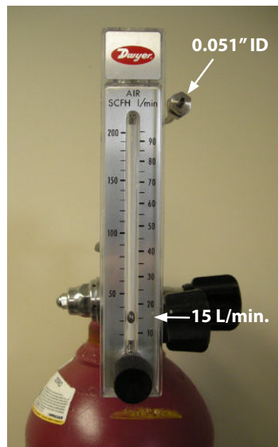
Figure 3: Further decreased flow through rotameter when loaded with a 0.051" ID orifice.
