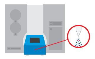
The coated blade with collected sample is coupled directly to a mass spectrometer through an interface. The sample is then ionized via electrospray ionization directly from the blade and analyzed by the MS *in seconds*. Direct-to-MS sample analysis dramatically reduces screening times.
