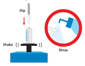
Analytes of interest are collected by the blade's coating. Larger, matrix-related compounds are not incorporated into the coating and are easily rinsed off prior to analysis.
