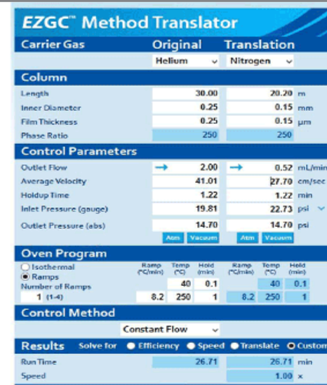
Figure 10: Screen shot of method translation showing the impact on parameters when changing column dimensions from 30m/0.25/0.25 and helium under speed optimized flow/velocity, to 20m/0.15/0.15 and using nitrogen. Operating nitrogen at 0.52 mL/min shows the same analysis time and the same programming conditions.
