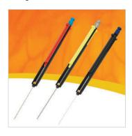
Our SPME product line is getting SMART—Restek now offers Smart SPME Arrows and Smart SPME fibers. The new Smart technology offers the same application, performance, and lifetime as the products you've come to rely on with the added feature of a smart chip that can keep track of parameters, ranges, and usage history.
