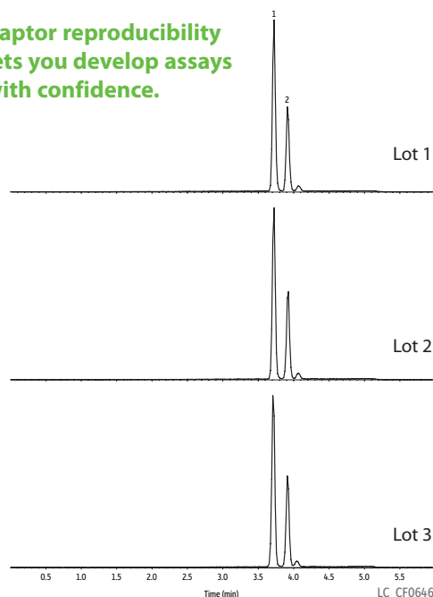
Figure 13: Raptor FluoroPhenyl columns have the selectivity and retention you need to quickly and easily separate compounds that coelute on a C18, such as the epimeric forms of vitamin D2 and D3 25-hydroxy metabolites.
