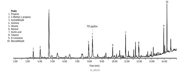
Column: Rtx-VMS, 60 m, 0.25 mm ID, 1.40 µm (cat.# 19916) with MXT low-dead-volume connector (cat.# 20536); Injection: on-column; Oven: Oven Temp.: 40 °C (hold 7 min) to 250 °C at 30 °C/min (hold 2 min); Carrier Gas: He, constant flow; Flow Rate: 2.0 ml/min; Detector: MS; Mode: Scan; Start Time: 8.80 min; Scan Range: 38 amu; Scan Rate: 226 scans/sec; Transfer Line Temp.: 250 °C; Analyzer Type: Quadrupole; Source Type: Extractor; Extracto
