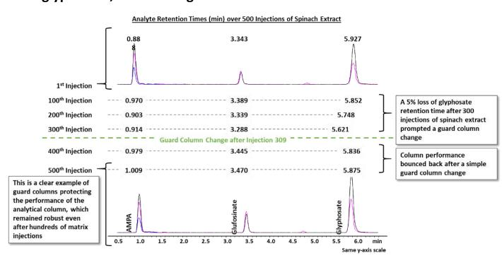
Fig. 6: Analyte retention over 500 injection. The data demonstrate a guard column protects and extends the column lifetime beyond 500
