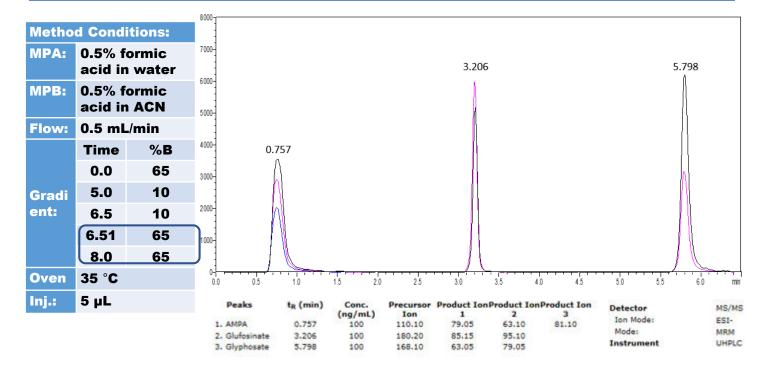
Fig. 3: LC-MS/MS separation of glyphosate, AMPA and glufosinate on a hybrid IEX/HILIC column (2.1x30 mm, 2.7 µm). Note the sharp peak shapes, fast equilibrium time (1.5 min) between runs, and short cycle time (8 min).
