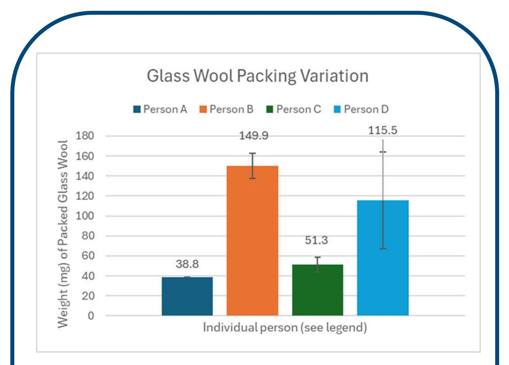
EPA method 1633 calls for the addition of silanized glass wool to be added at half the height of the WAX SPE cartridge barrel. With no specific weight given for the silanized glass wool, this can create inconsistencies in the amount packed in cartridge from cartridge-to-cartridge and technician-to-technician. The graph above demonstrates the variability in silanized glass wool being packed with 4 individuals packing 5 SPE cartridges per EPA guidelines.
